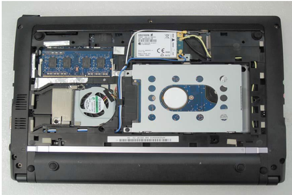
GSM/3G module installed in a netbook computer
