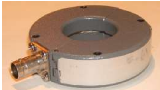
Fischer F-61 Listening 1 \text{ MHz} \leq F \leq 1 \text{ GHz}
