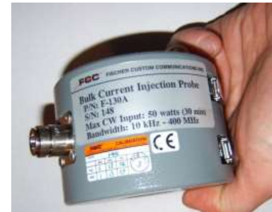
Fischer F-130x Injection 10 \text{ kHz} \leq F \leq 400 \text{ MHz}
