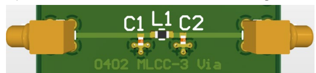
Figure 4: Measuring channel with 0403 MLCC and 3 vias each at the GND pad
