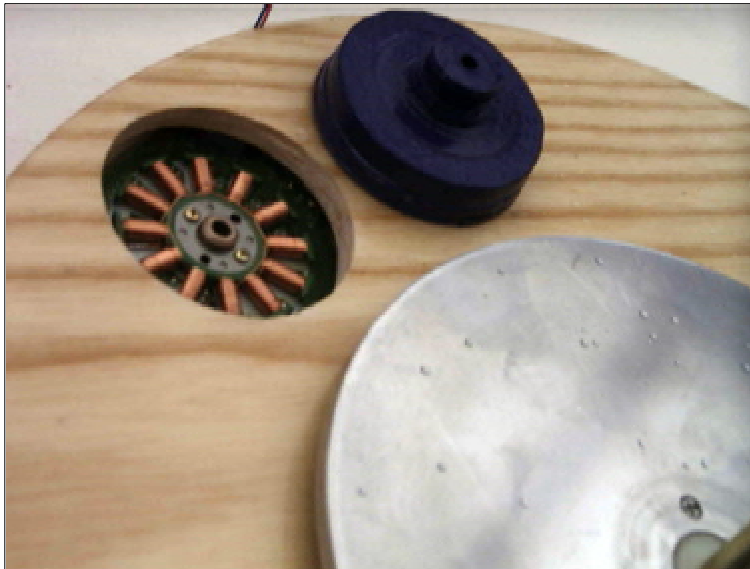
I mounted the floppy motor recessed about 10mm under the wood... This is a 33rpm pulley.
