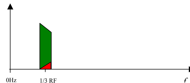
Figure 2-10 RF-mixer output with the use of a tracking filter. Image is suppressed.
